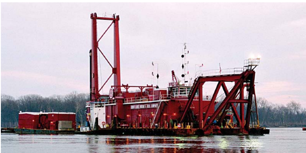
Figure 14. Cutterhead dredge California (courtesy of Great Lakes Dredge and Dock Company).
