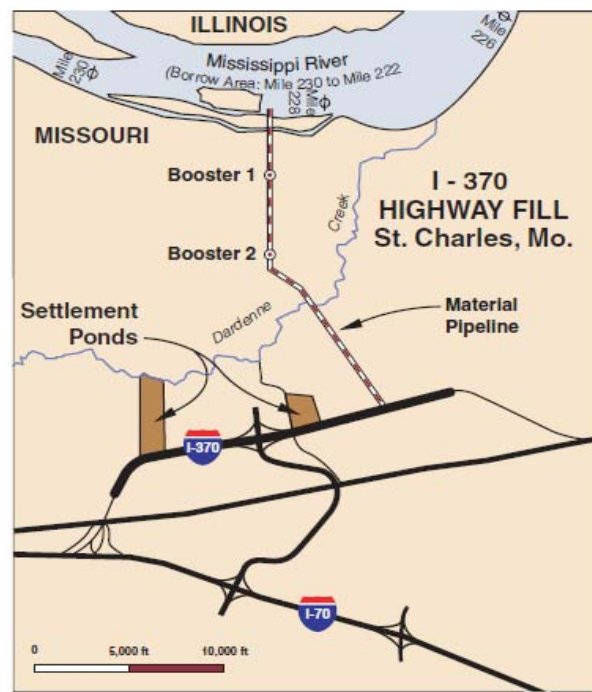
Figure 13. I-370 Highway Fill St. Charles MO site map (courtesy of Great Lakes Dredge and Dock Company).
