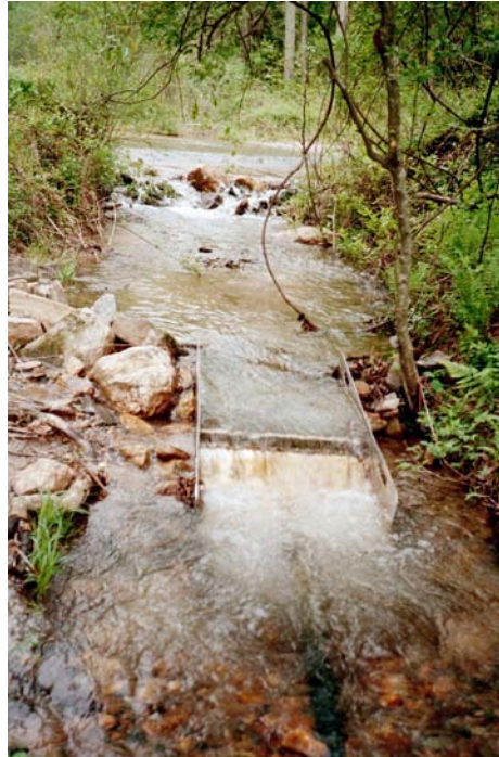
Figure 49. A bedload Collector™ installed in a stream (courtesy of Streamside System®).
