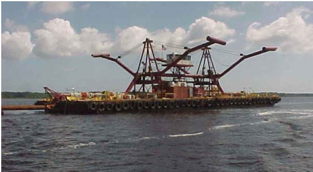
Figure 9. Spider barge connected to hydraulic pipeline dredge.
