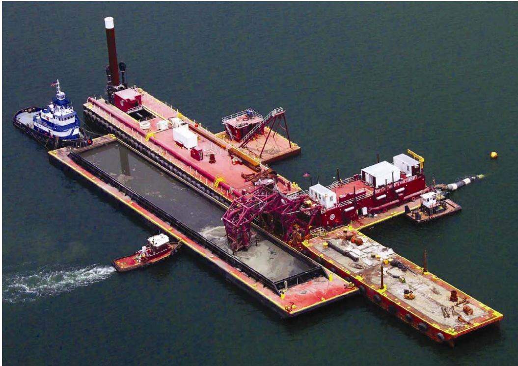
Figure 10. Hydraulic unloader (courtesy of Great Lakes Dredge and Dock Company).
