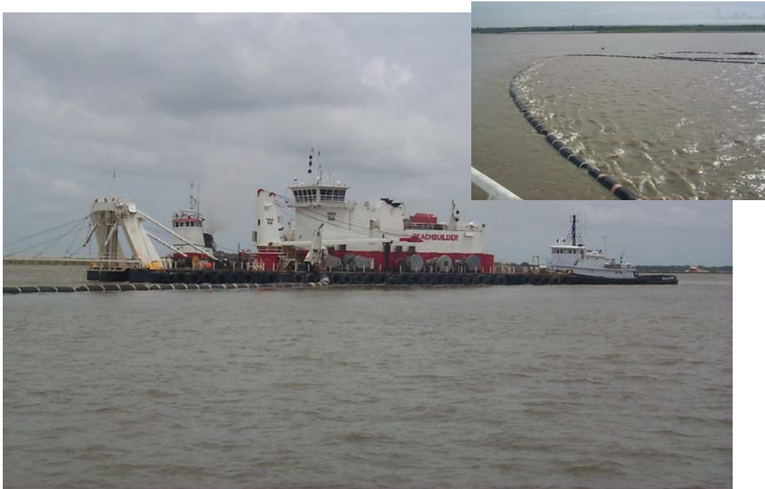
Figure 40. Dustpan dredge Beachbuilder and flexible floating line (insert) used to effectively dredge entire width of Mississippi River navigation channel.
