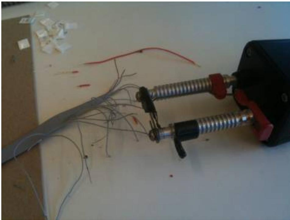
Figure 23. Stripping the sheath off wires of the 20-pin C2B data cable
