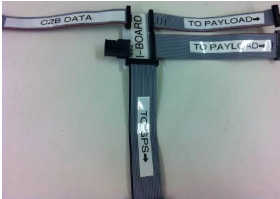
Figure 27. Pseudo PCB I-board with C2B data and power (left), payload cables (right), and GPS cable (bottom)
