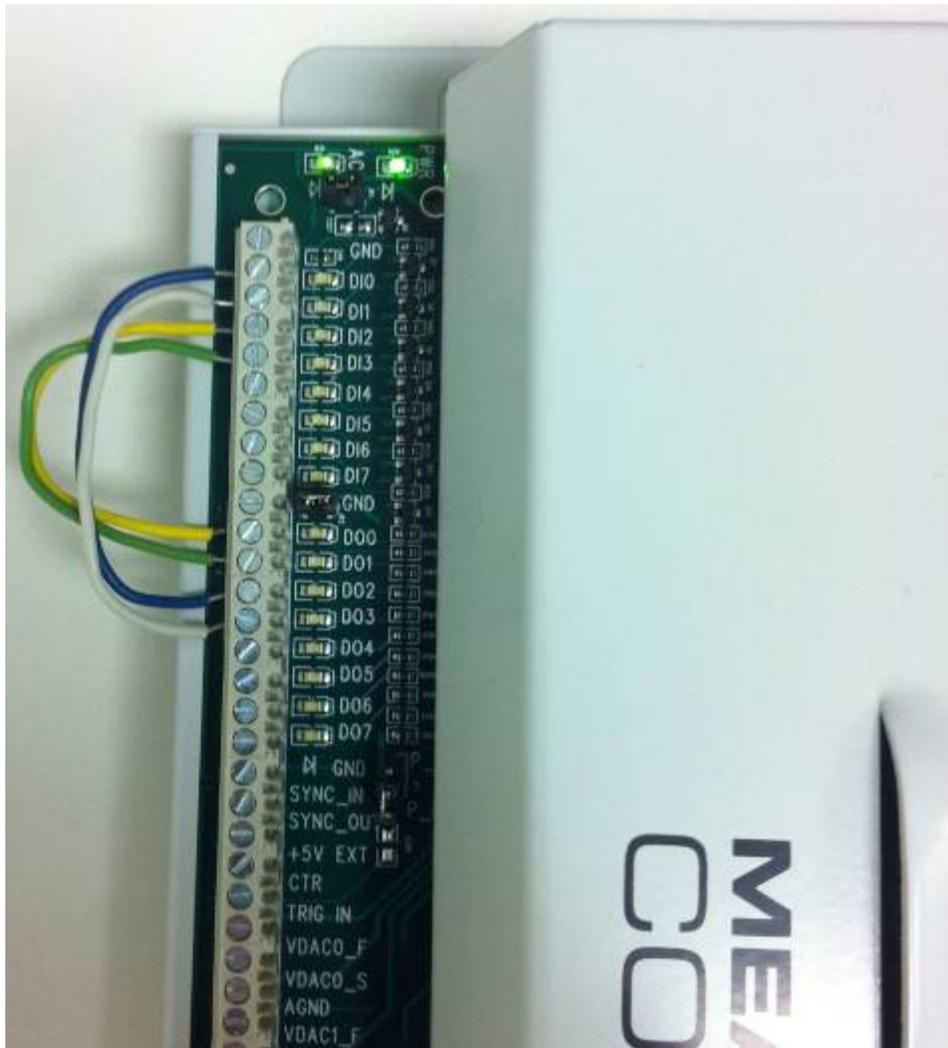
Figure 37. MCC DAQ controlled by C2B interface GUI, not using DIO
