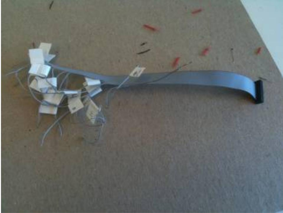
Figure 24. Labeling the wires of the 20-pin C2B data cable
