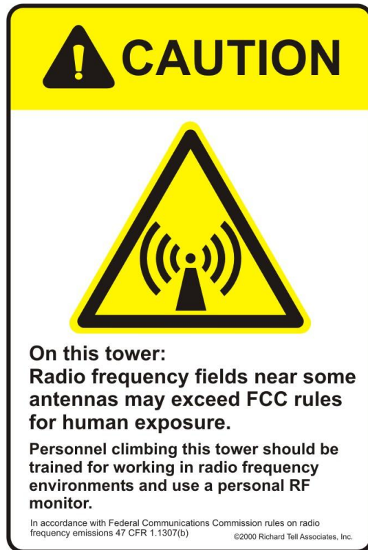
Figure 10-8. Example of an RF Caution sign designed to alert personnel to localized RF exposure on antenna towers following IEEE C95.2-1999.
