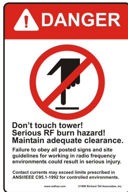
Figure 10-3. Example of a DANGER RF alerting sign used to advise of potential RF burn hazards.
