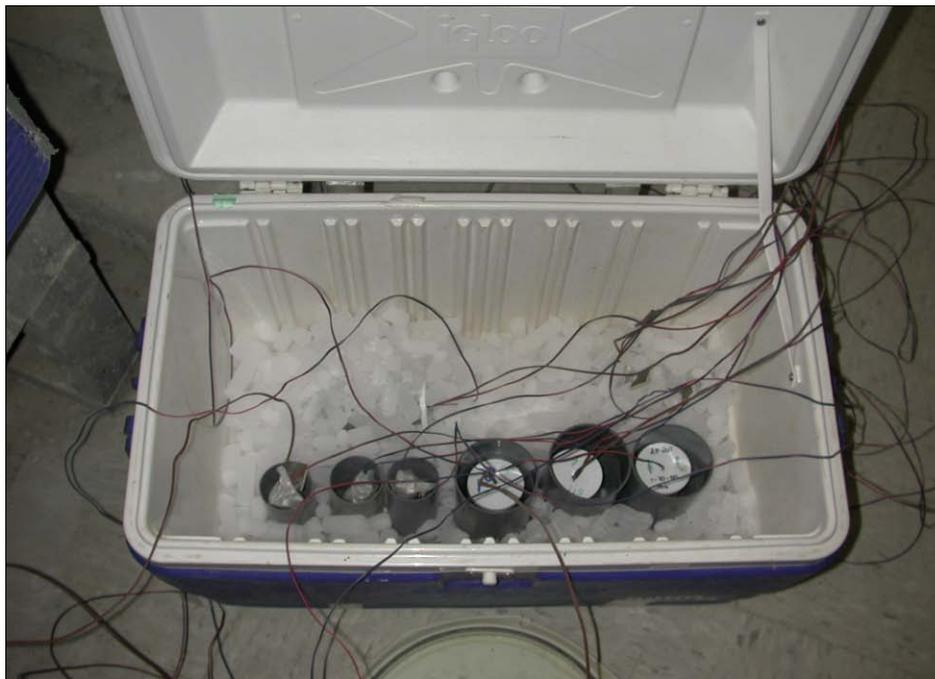
Figure 10. An example of the freeze-point field setup showing samples of fresh concrete with embedded temperature sensors freezing in the portable cold chamber.
