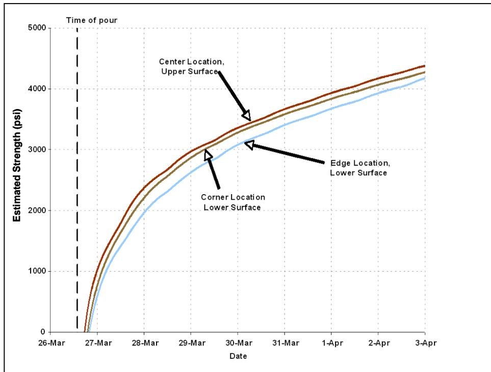
Figure 19. Estimated compressive strength development for Mixture 3 in Section 5 at upper center, lower edge, and lower corner locations in structure.
