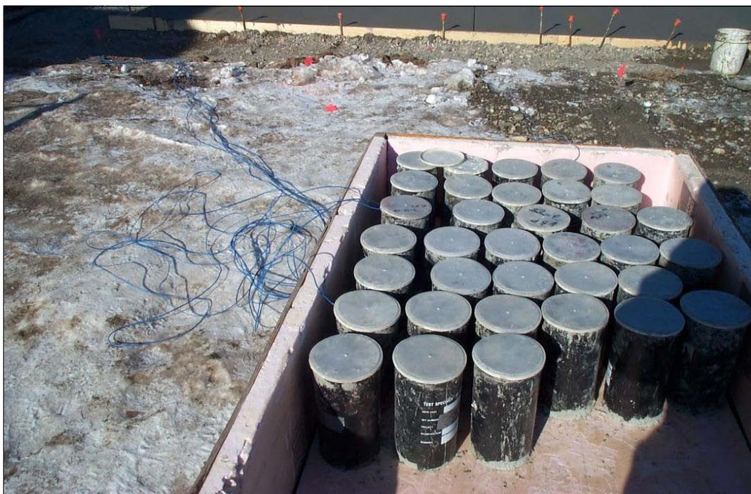
Figure 6. Field-cured cylinders kept onsite in insulated box.
