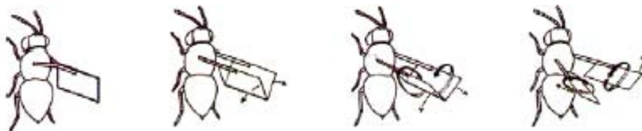
Figure 1.2 Clap and fling mechanism for housefly (Ref. C P Ellington, 1999)
