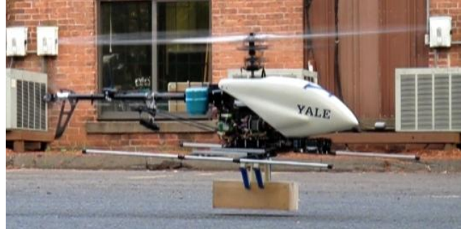
Fig. 1. Yale Aerial Manipulator capturing an object while hovering.
