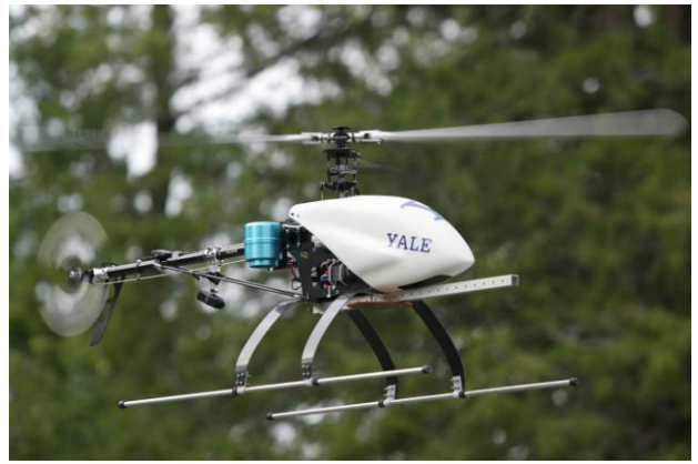
Fig. 10. Yale Aerial Manipulator with payload rail and fixed gear.
