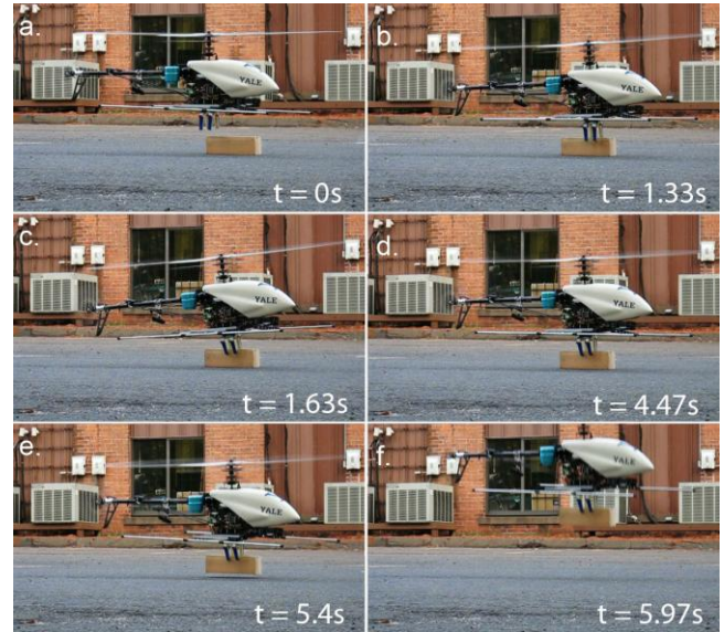
Fig. 17. Grasp and retrieval of a block while in hover
