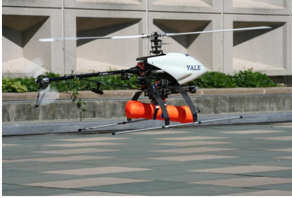
Fig. 2. Yale Aerial Manipulator with gripper and fixed gear.
