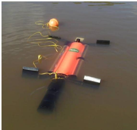
**Figure 8: Transphibian with ADCP and Environmental Sensors Installed during Initial Field Tests**
