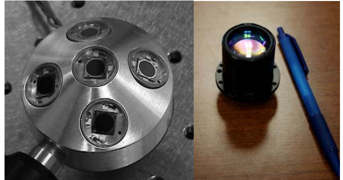
Figure 2: a) Corner cube MRR array b) Cat’s eye MRR.
