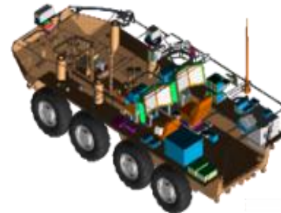
MGV With Embedded UGV Control
