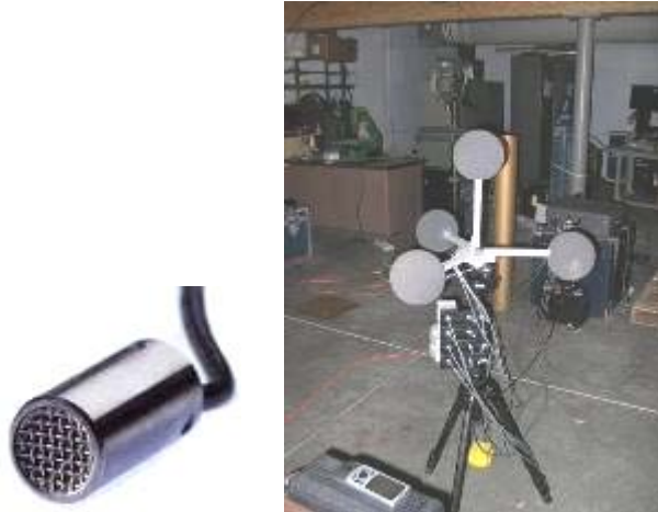
Figure 1. Single microphone and an array (tetrahedral) of microphones with windscreens.
