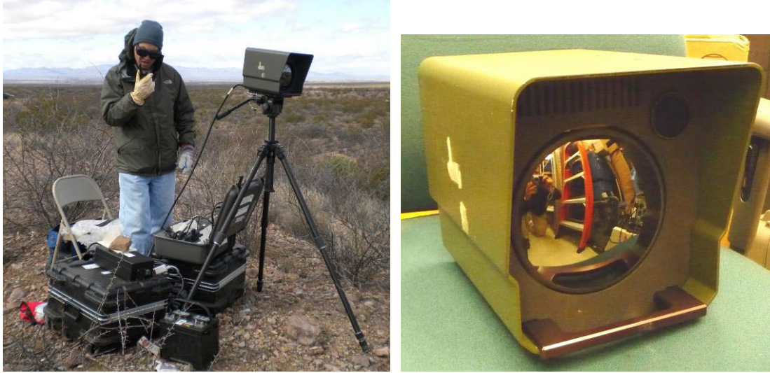
Figure 11. Picture of emplaced TRSS dual imager and ARL data recorder, plus a close-up shot of imager.
