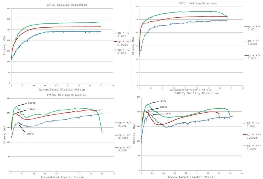
**Figure 2. Cyclic hardening curves for specimens tested parallel to the rolling direction of the parent plate. Note that the abscissa on each plot is accumulated plastic strain, and not cycles, to allow for comparison between different strain amplitudes.**
