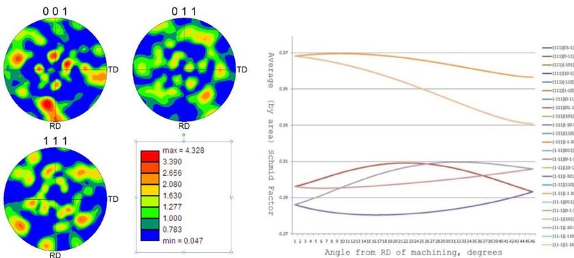
**Figure 1. Pole figures for the material as tested, and average Schmid factors for each slip system calculated from the OIM data. All slip systems have been plotted as a mathematical check despite the overlay between many systems.**
