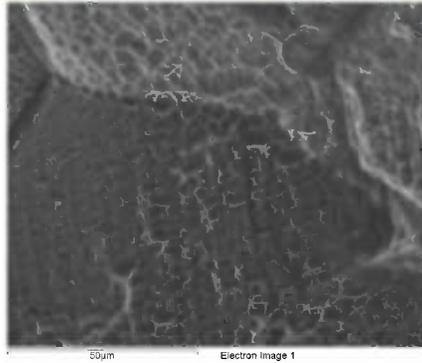
**Figure 5. Scanning electron micrograph, showing ductile dimples and fatigue striations on the fracture surface of a specimen machined at 45° from the parent plate and tested to failure (800 cycles) at  $\epsilon_p = \pm 0.001$ , 1 Hz, 200°C.**
