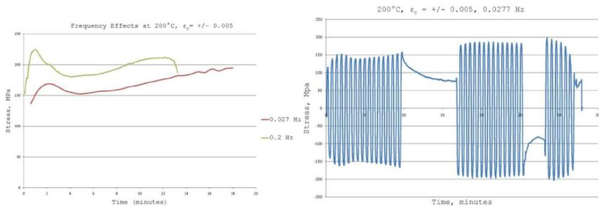
**Figure 4. Frequency effects and recovery behavior during holds at 200°C. Note the change in the abscissa to time from accumulated plastic strain to allow comparison of hardening effects. Samples sectioned from parent plate parallel to the rolling direction.**
