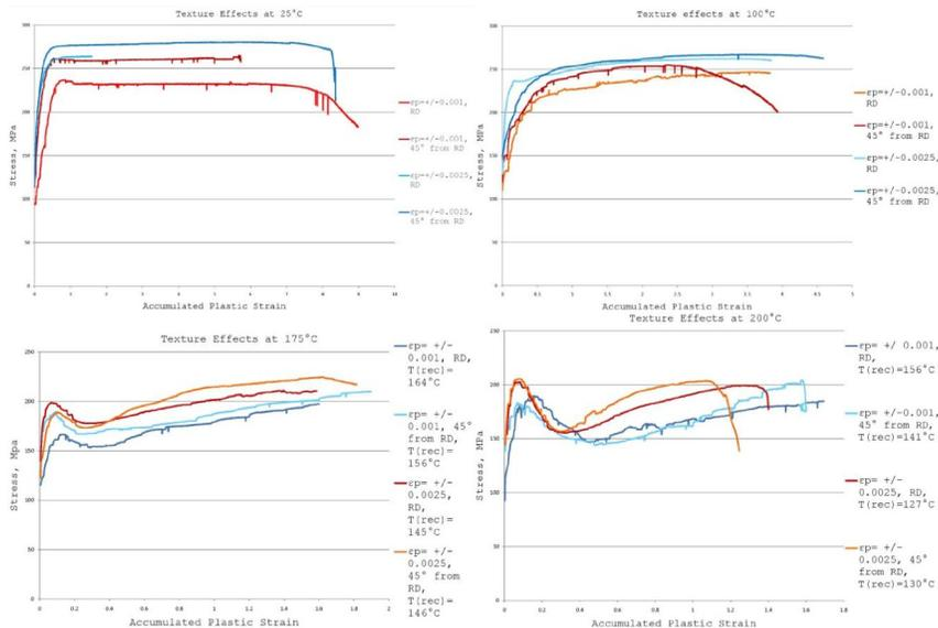
**Figure 3. Cyclic hardening curves for specimens machined at  $45^\circ$  from the rolling direction of the parent plate. Temperatures corresponding to the early peak are listed in the legend for specimens tested at  $175^\circ\text{C}$  and  $200^\circ\text{C}$ .**
