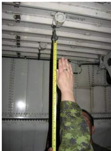
Figure 3 Measurement of reach for the SKAD arming cables.
