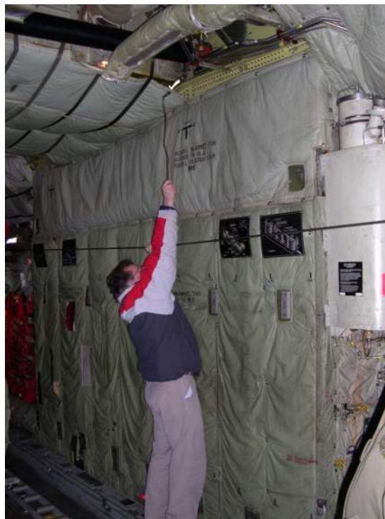
Figure 11 Reach for bleed air valve control (highlighted)
