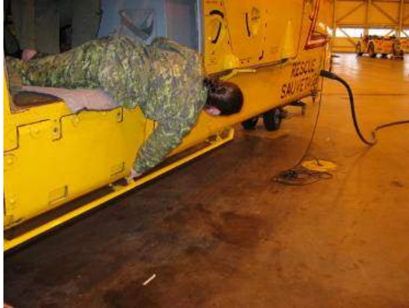
Figure 8. Landing area monitoring from the cargo hold
