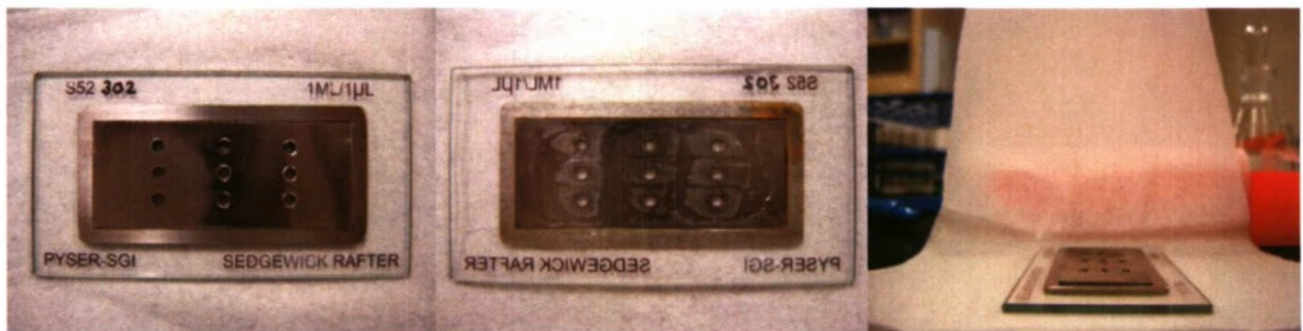
Figure 3. Photographs of a "custom" sample well tray designed by NRL. This approach may provide the ability to match well geometry to the microscope-camera system's imaging capabilities.
