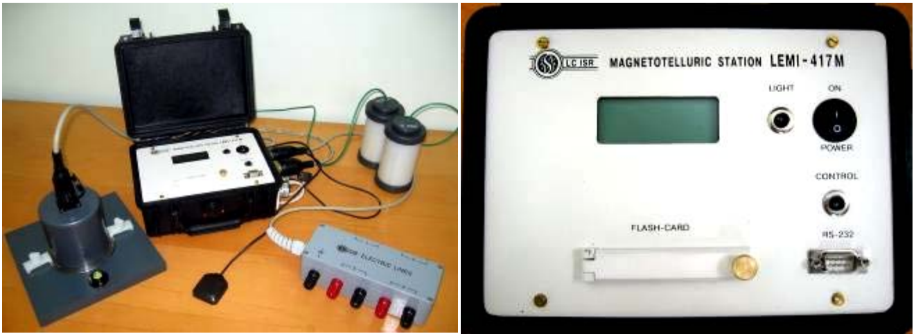
Figure 1 Magnetotelluric station LEMI-417 set (left) and its front panel (right)
