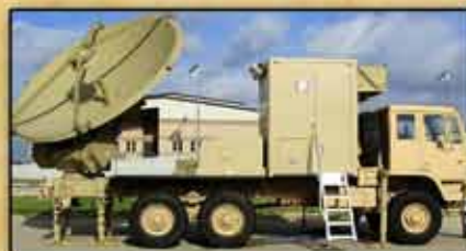
The tactical "hub" terminal of the Joint Network Node
