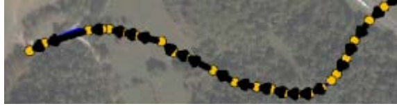
Figure II.1: A curved line sampled from user input. The yellow circles represent the sampled waypoints. Note that many of these waypoints may not be necessary to accurately describe the line.
