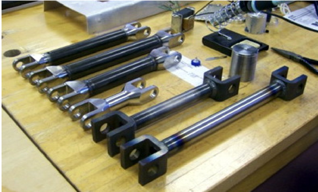
Figure 15. Photograph of the four sets of test samples generated by alternative manufacturing processes.
