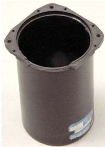
a) Original part with damage at the flange
