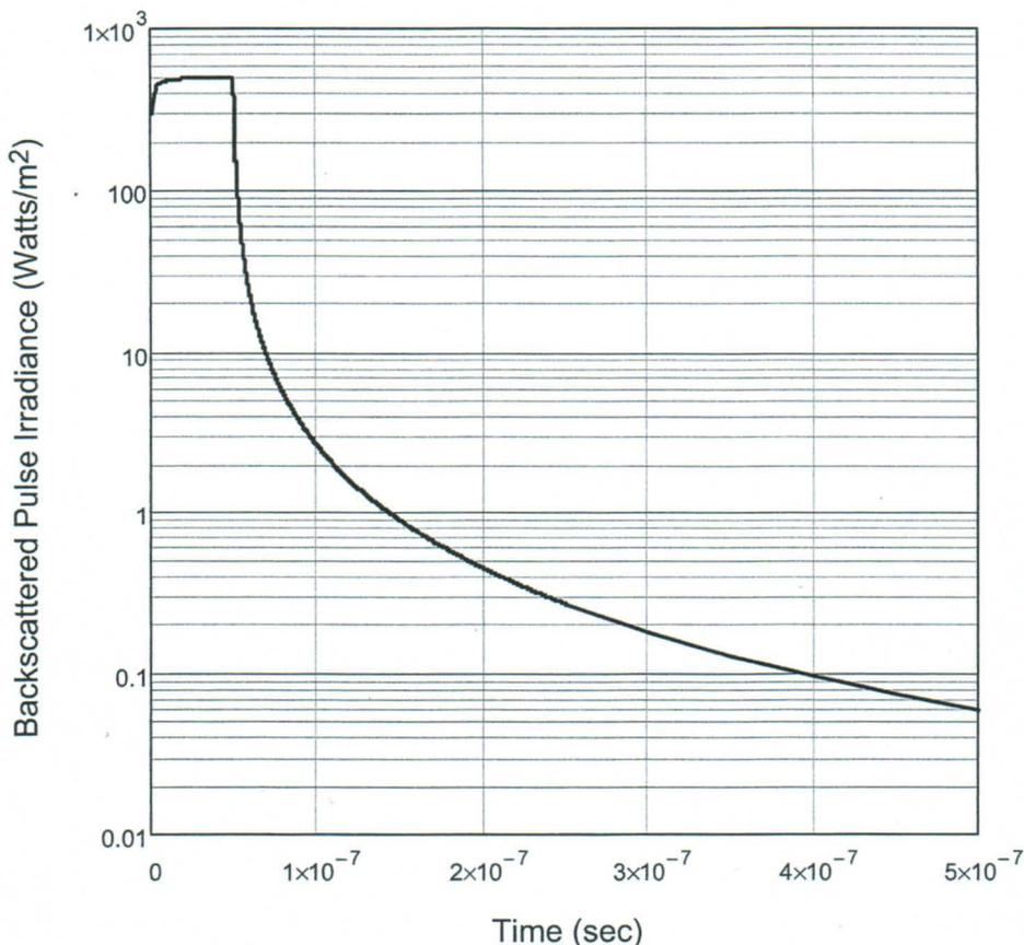
**Fig. 2.** Typical backscattered irradiance waveform on the aperture plane produced by a propagating laser pulse.
