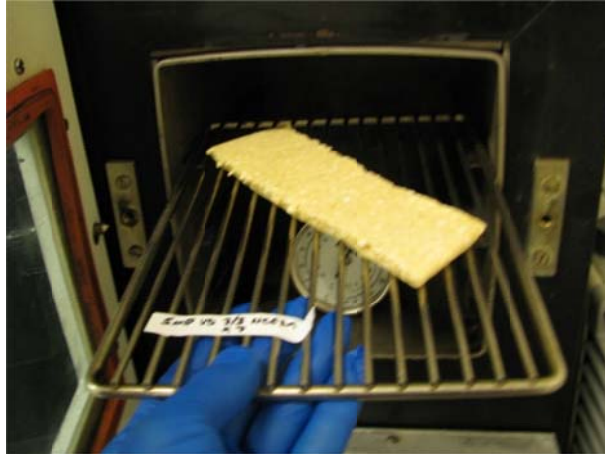
Figure 3-12: Bar being placed into vacuum chamber before freeze drying
