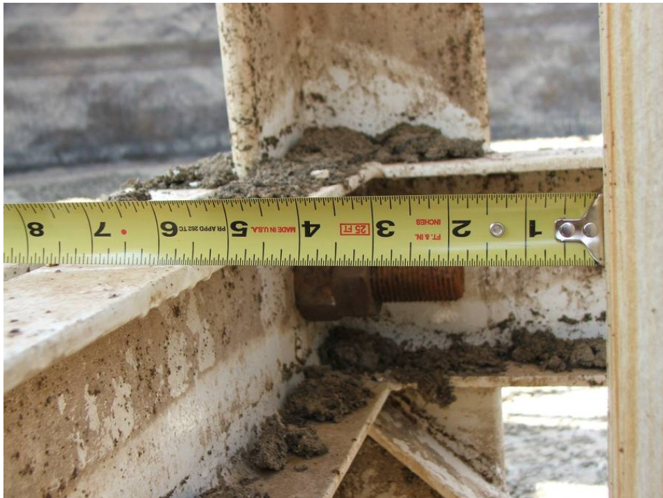
Site Photo 5. Main shaft was positioned approximately 5 5/8 inches from the static frame.
