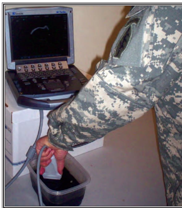
Figure 2: Fracture detection of the opaque study model via the SonoSite M-Turbo portable ultrasound.
