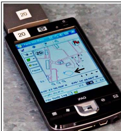
Figure 1. Field GIS Hewlett-Packard personal digital assistant with US GlobalSat GPS, and Farm Works field GIS software shown mapping a mosquito breeding pool identified by black arrow.
