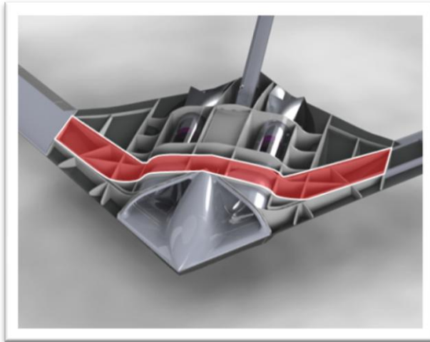
Figure 14 - Location of Unidirectional Reinforcement in Fuselage Skins (Top Skin Shown in Red)
