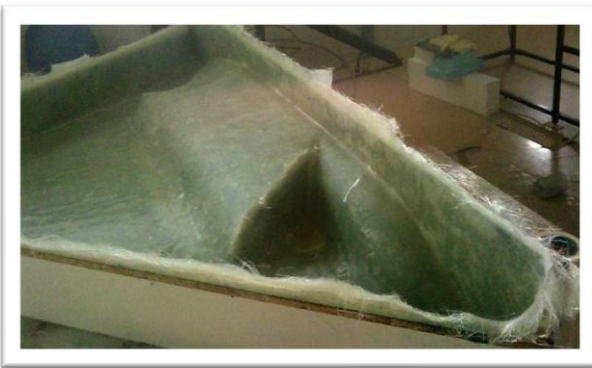
Figure 11 – Fiberglass Female Mould Curing on Plug
