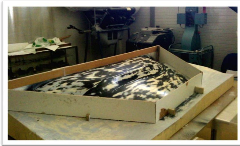
Figure 10 - Finished Plug with Vertical Walls Built Around Perimeter
