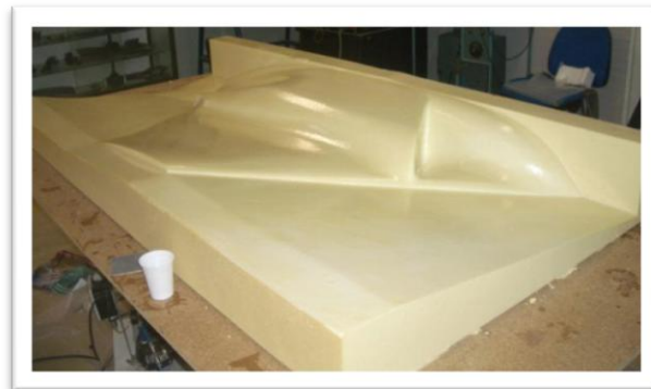
Figure 9 - Plug after Application of fiberglass Layer
