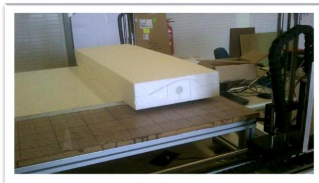
Figure 18 - CNC Hot Wire Cutting Wing Profile
