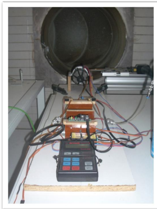
Figure 2 - Turbine Engine Test Stand to be used for determining TSFC of Jetcat Engines
