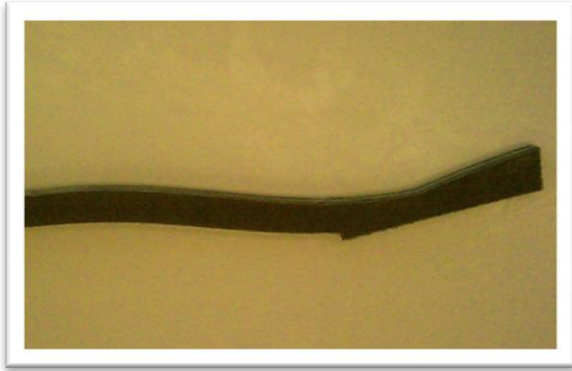
Figure 19 – End of Rear Wing Shear Web that Joins with Forward Wing
