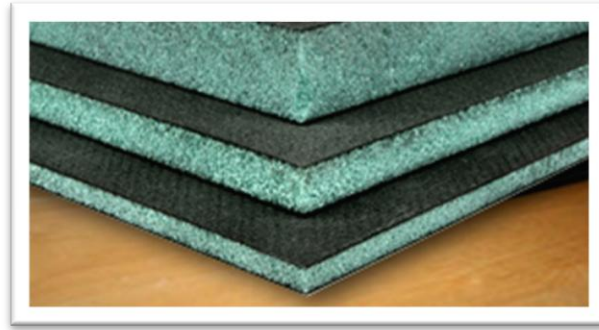
Figure 3 - Laminate Sheets Produced using VARTM
