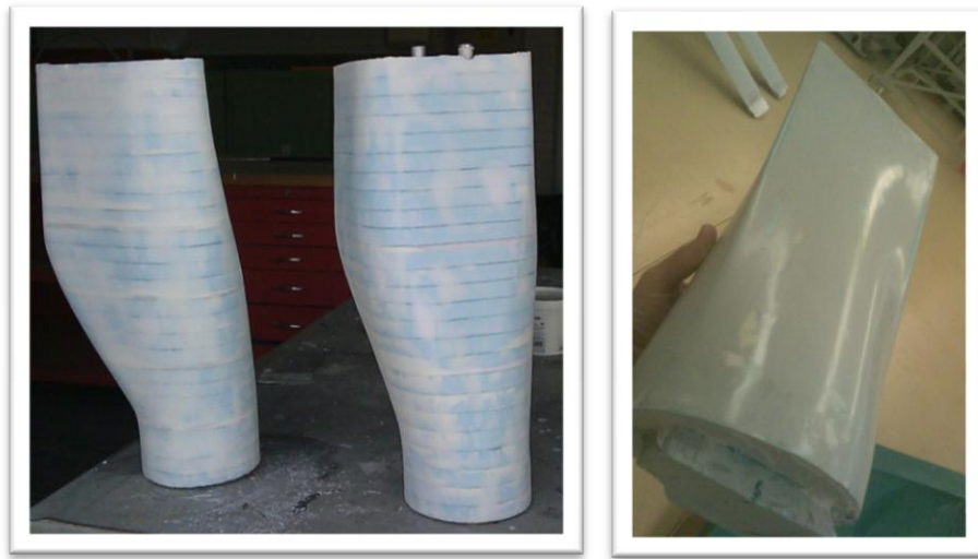
Figure 24 - Male Plugs Used for Producing Air Intake Skins (left) and Outlet Skins (Right)
