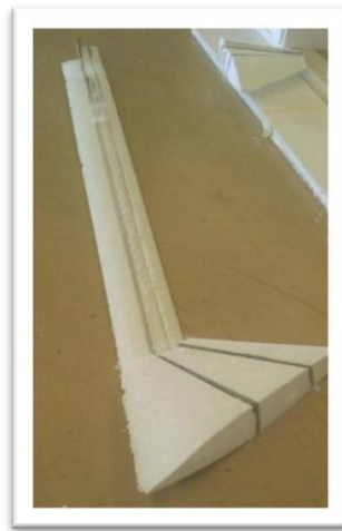
Figure 21 - Aft Wing Foam Core Ready for Vacuum Bagging
