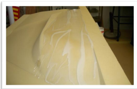
Figure 8 - Application of Micro Slurry to Seal Plug
