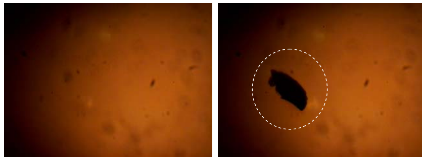
Figure 6 Video microscope images of thin Au films with less than 300 nm thickness. Left: Before laser exposure. Right: Laser induced surface damage was observed with high peak power pulses and at shorter laser wavelengths.
