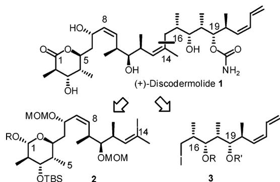
**Figure 1.** First disconnect for the retrosynthesis of (+)-discodermolide.
