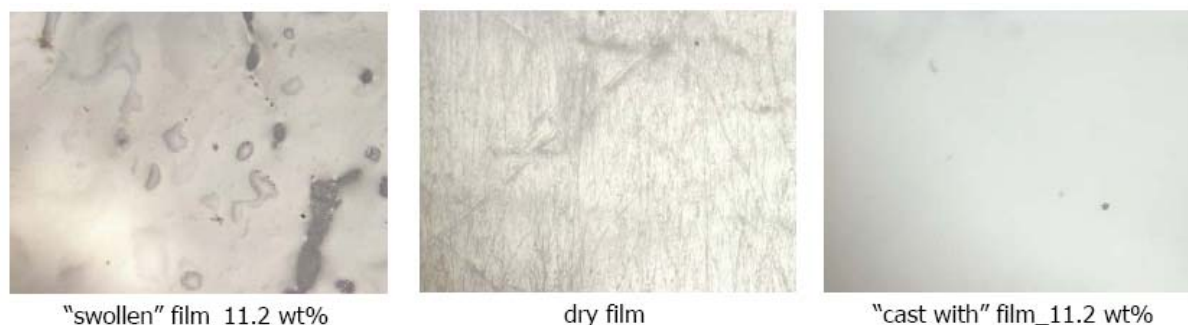
Figure 17 Optical microscopy images of a dry zwitterionomer film and two zwitterionomer/IL composite films prepared via the “swollen” method and the “cast with” method.
