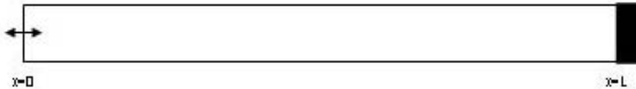
Figure 2: Impedance Tube. The left edge consists of a piston vibrating with a prescribed velocity. The right edge has a known impedance.
