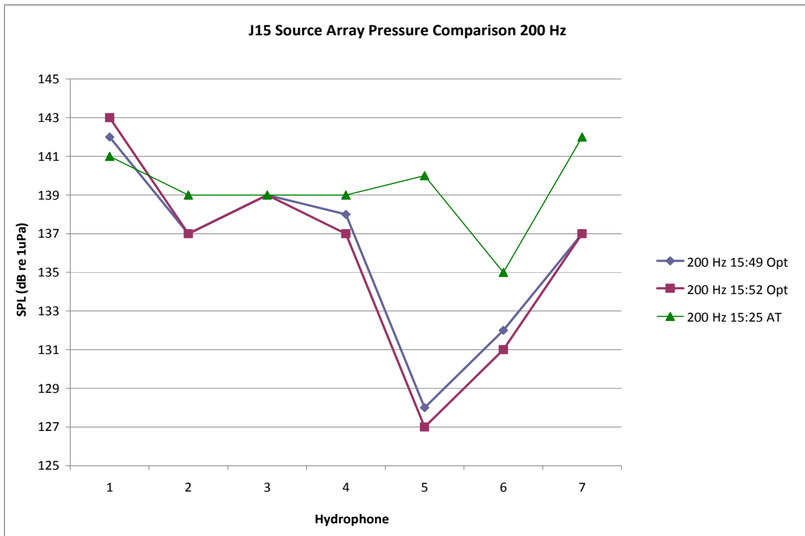
Figure 16: Sound Pressure Level at each hydrophone with phasing via the Optimal Phase Search method and the classic array theory at 200 Hz for the J15 Source Array.
