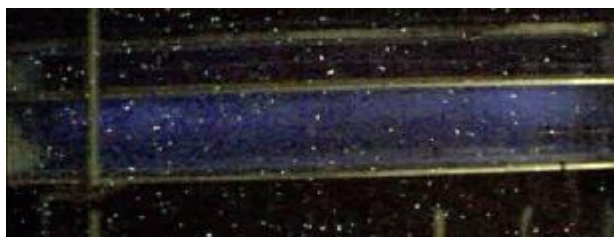
Photo 1 Fig.24 Photos of a luminescence of air under the influence of the electron beam in the volume of the experimental chamber, at various values of a current in the magnetic coil of the scanning system . (The current I_1 the the photo (1) is << than the current I_2 at the photo (2)).
