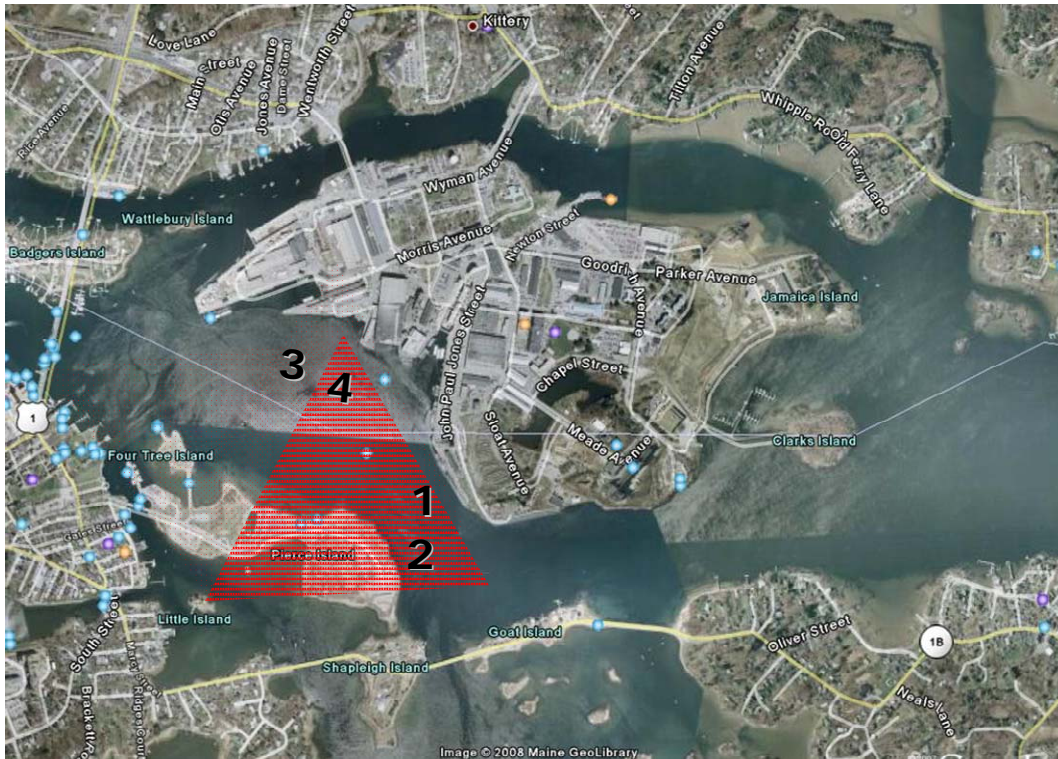
Figure 2. Planned installation for the Portsmouth Navy Shipyard. The first two nodes (1,2) will be placed side-by-side on the southern point of the island covering the channel to the west, while the other 2 nodes (3,4) will be placed so as to cover the same area from the northwest. In this fashion a there will be a large region of coverage for developing bi-statics.
