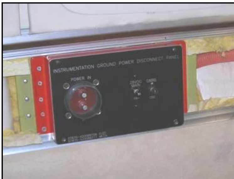
Figure B1. Instrumentation Ground Power Disconnect Panel
