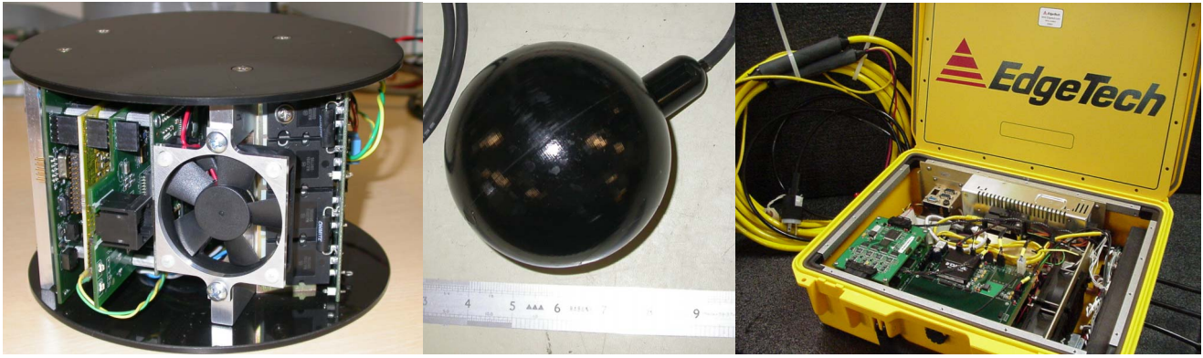
Figure 1. Completed Underwater Modem Electronics Stack (left), Jetasonic H320 Source Transducer (center) and Portable Topside Unit (right) for the Very High Bit Rate Acoustic Modem.
