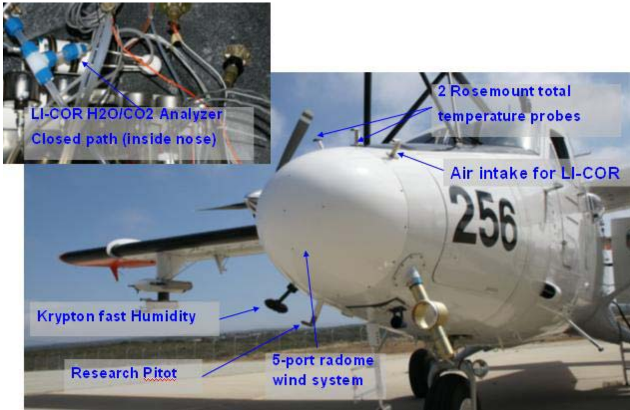
Figure 1: UCI Turbulence instrumentation on the CIRPAS Twin Otter for POST and VOCALS-REx field experiments in 2008.
