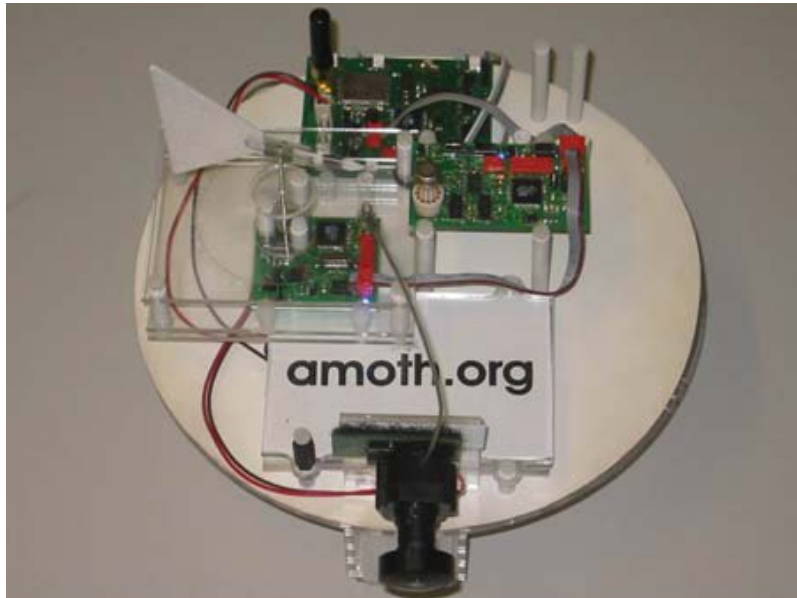
Figure 29. The artificial moth robot (diameter = 20 cm) (Pyk et al., 2006).
