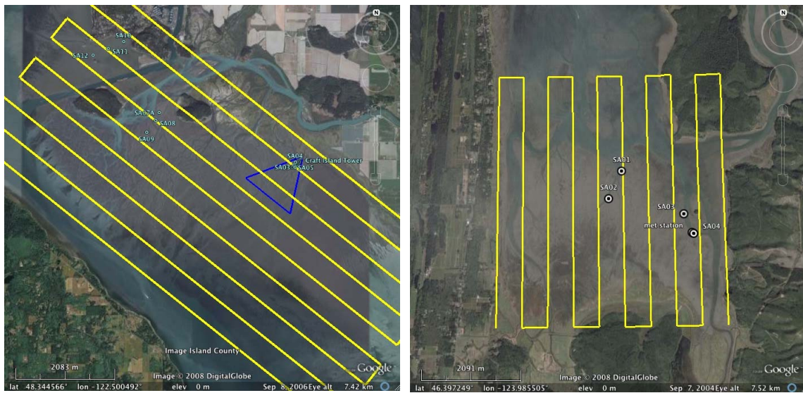
Figure 2. Google Earth images showing instrument locations (dots), overflight tracks (yellow lines), and tower field of view (blue triangle) during FY08 field experiments on the Skagit (left) and Willapa (right) Flats.
