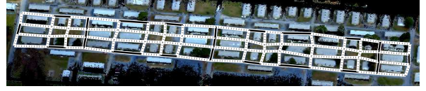
Fig. 2. (a) We represent the prior map as a graph where edges (white lines) denote the roads and vertices (stars) denote the road intersections. (b) Dotted and solid lines represent the CPP solution and are super-imposed on the above graph. Dotted lines denote edges that are traversed once and solid lines denote edges that are traversed more than once.
