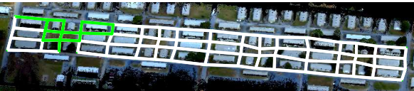
Fig. 7. The final path is replanned for the updated graph. This path starts at the node where the previous traversal ended.
