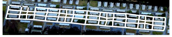
Fig. 3. During traversal of the CPP solution, the robot discovers that the third edge in the path is missing and ends the traversal. Dotted lines denote edges that are traversed once and solid lines denote edges that are traversed more than once.
