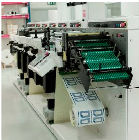
Figure 2.7. A roll-to-roll printing machine in Acreo's Printed Electronics Laboratory.
