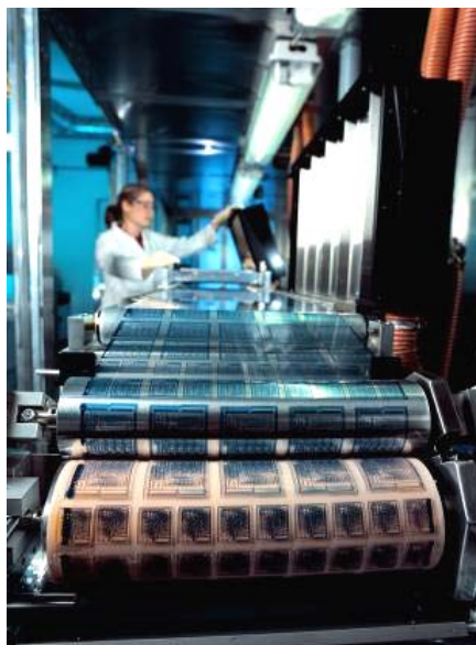
Figure 6.7. Wide-web roll-to-roll solution processing manufacturing platform (courtesy of PolyIC).
