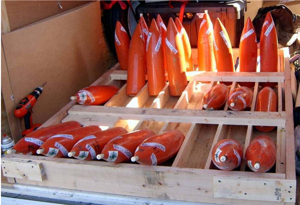
Figure 15. Surrogate 5"/38 projectiles used in UXO Mobility Model field demonstrations.
