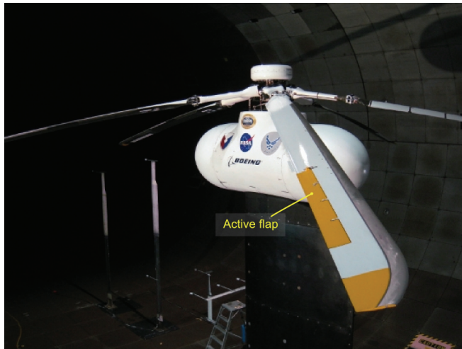
Figure 1. Boeing-SMART rotor with active trailing-edge flaps in the NFAC 40- by 80-Foot Wind Tunnel.
