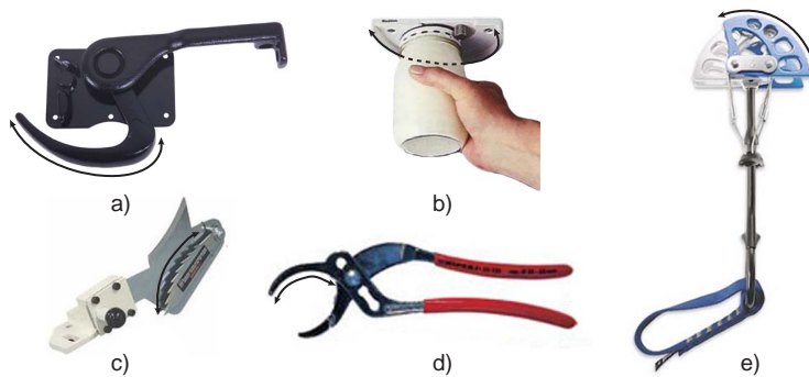
Fig. 2 Curved shapes used in: a) Truck door lock; b) Jar opener; c) Anti-kickback device for table saw; d) Pliers; e) Climbing cam
