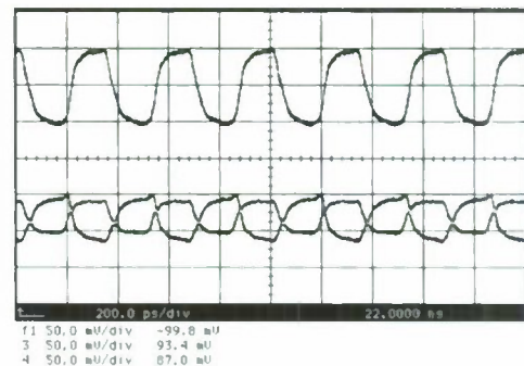
Fig. 7. Measured waveforms of the DAC output (one bit is toggling at 6 Gb/s): differential (top) and single ended (bottom)
