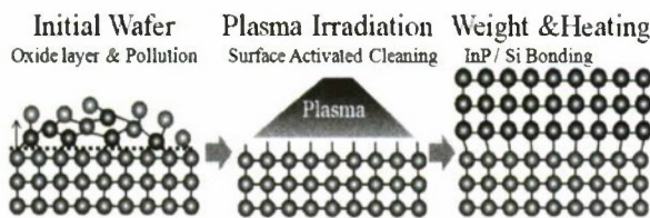
Fig. 1 Surface activated bonding processes.
