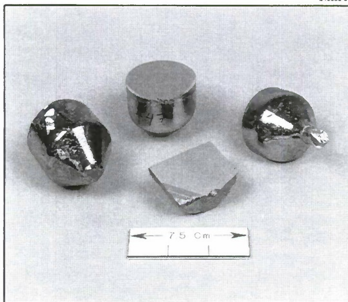
Figure 3-2. Four InP boules grown by VGF method. Several twins are noticeable in the center front boule.
