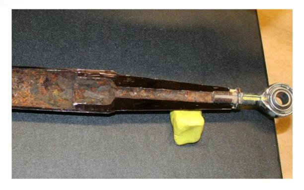
A Category I Quality Deficiency Report (QDR) investigation of the FWD Fast Rope Insertion Extraction (FRIES)/External Recue Hoist support rod (P/N LEX-1583-05), consisting of microscopic, ultrasound, and metallurgic examination revealed severe corrosion of the inside surface of the rod. Subsequent investigation of additional ship sets revealed several support rods within the FWD FRIES/External Rescue Hoist truss assembly exhibiting similar corrosion.
