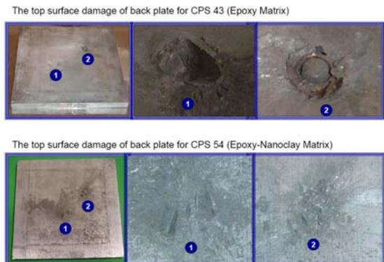
(b) The top surface damage of back plates
