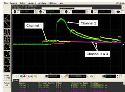
**Figure 15** Response signals from the blast tube test
