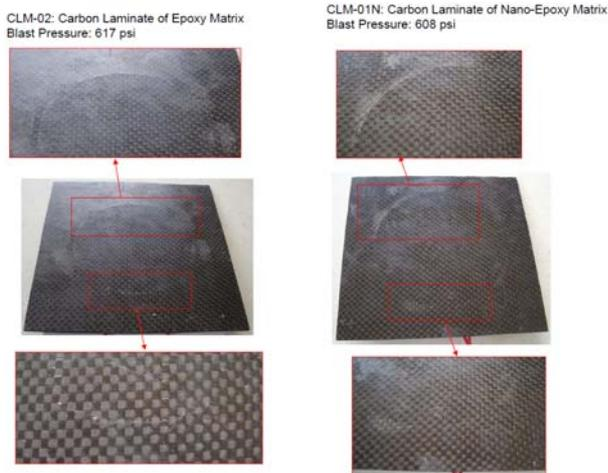
**Figure 17** Comparison of test results for carbon fiber laminates with pure epoxy resin (left) and nanoclay-reinforced epoxy resin (right).
