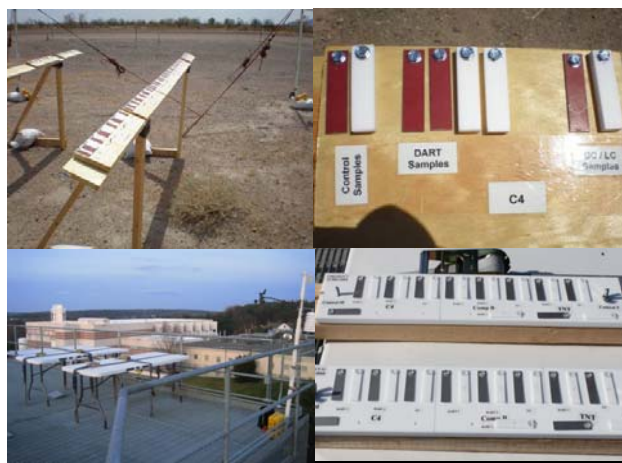
Fig 1. Photos of the Yuma Proving Ground test area and the test panels (top) as well as the Lexington, MA, test area and coupons mounted on Teflon® boards (bottom).
