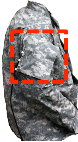
Fig. 8: Patch antenna (red box) design shown attached to the shoulder of an army-issued jacket using a hook and loop connector.
