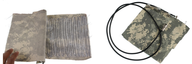
Fig. 6: Left) Picture of the prototype polypyrrole antenna with the upper layer peeled off and middle feed layer exposed. Right) The prototype with all the layers along with the TNC connector.
