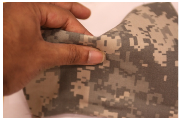
Fig. 7: The patch antenna device pinched to illustrate the flexibility of the overall design.
