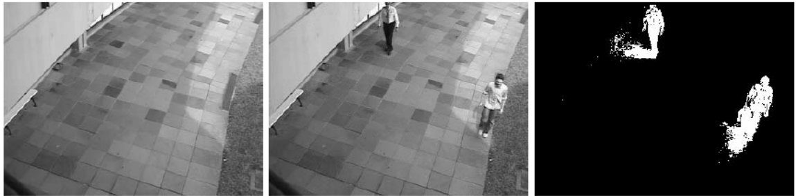
Figure 4. Background subtraction process, background model (left), input frame (center) and foreground extraction (right).
