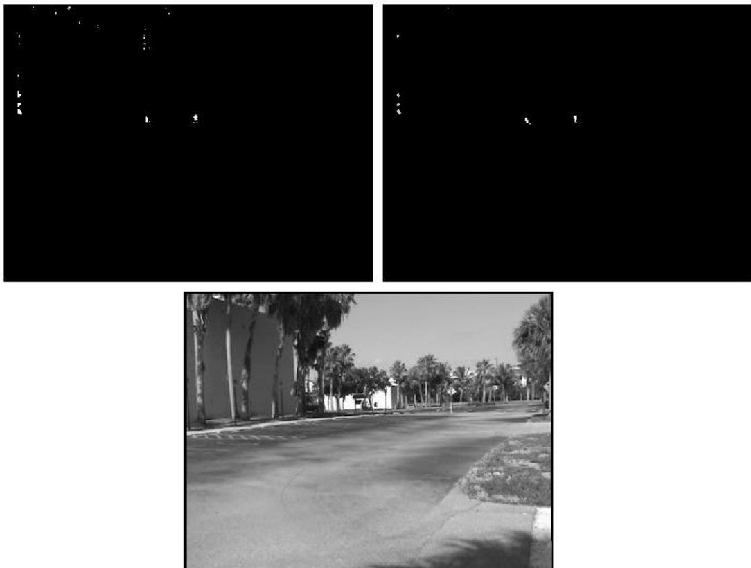
Figure 40: Grayscale image (bottom), background subtraction algorithm (top-left), and morphological filter output (top-right).
