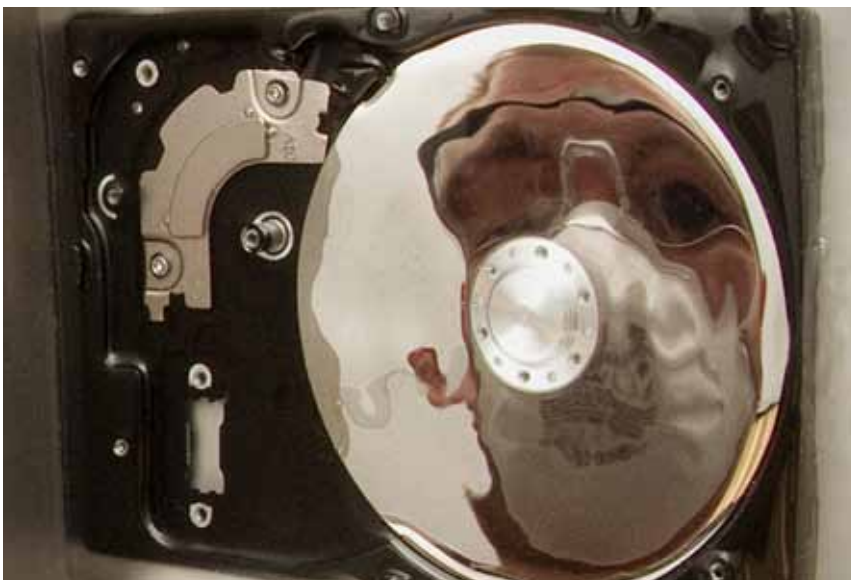
The reflection of senior forensic technician Scott Lalliss appears on the highly reflective disk of a hard drive undergoing sonic cleaning at the Defense Computer Forensic Laboratory in Linthicum, Maryland. Here, a 91-percent alcohol, 9-percent water solution produces bubbles that gently move dirt and other organic matter away from the disk. The surface requires careful handling to prevent damage and thus preserve data that may be valuable evidence for an investigation.
