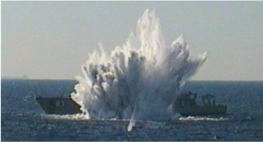
Figure 3: UNDEX Shock test of HMAS Hawkesbury, 1999 [16]
