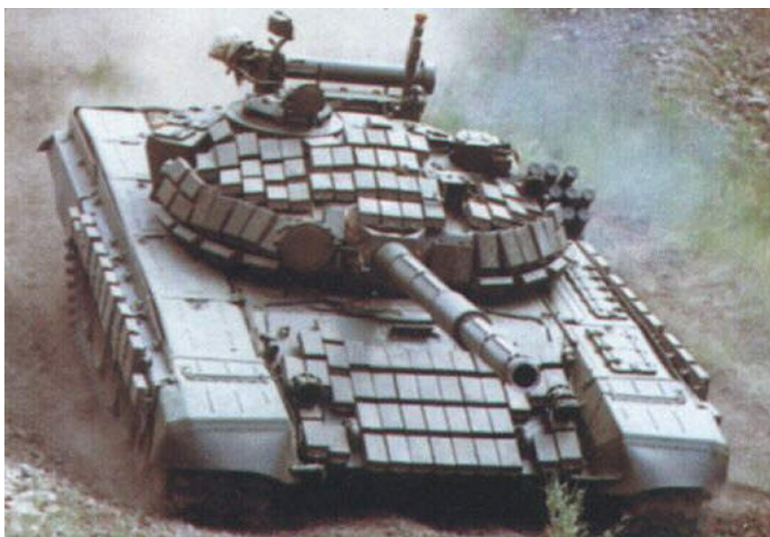
Figure 7: Example of explosive reactive armour as applied to a tank [31]
