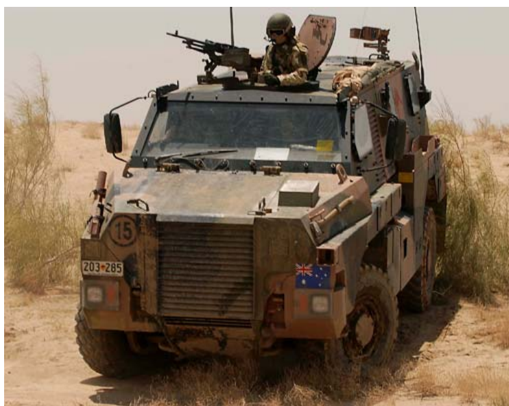
Figure 6: Australian Bushmaster infantry mobility vehicle with transparent armour windscreen and side windows [29]
