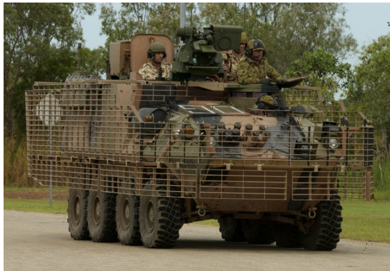
Figure 5: Australian Service Light Armoured Vehicle (ASLAV), showing examples of metallic (vehicle hull) and spaced (bar) armour [27].
