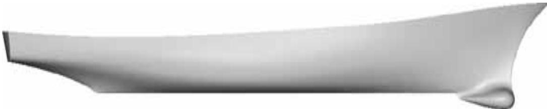
*Figure 1. Grey scale image of the DTMB model 5415 geometry*
