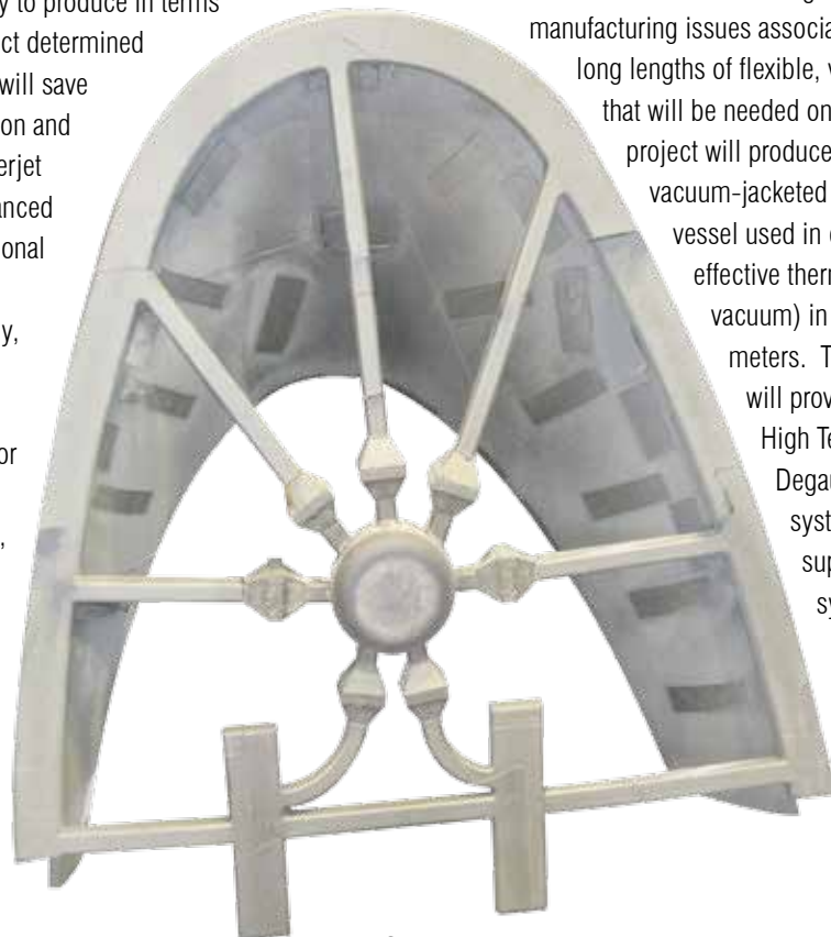
Marinette Marine Corporation is implementing a near-net-shape cast waterjet inlet edge on LCS that will reduce labor hours in fabrication and installation.
