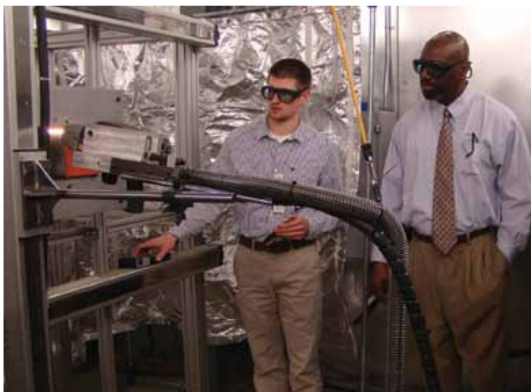
NMC is evaluating and developing laser coating removal processes in two current projects to reduce costs and labor over more traditional methods of coating removal. Pictured are Gerred Price, mechanical engineer, and Greg Woods, NMC program officer. CTC photos
