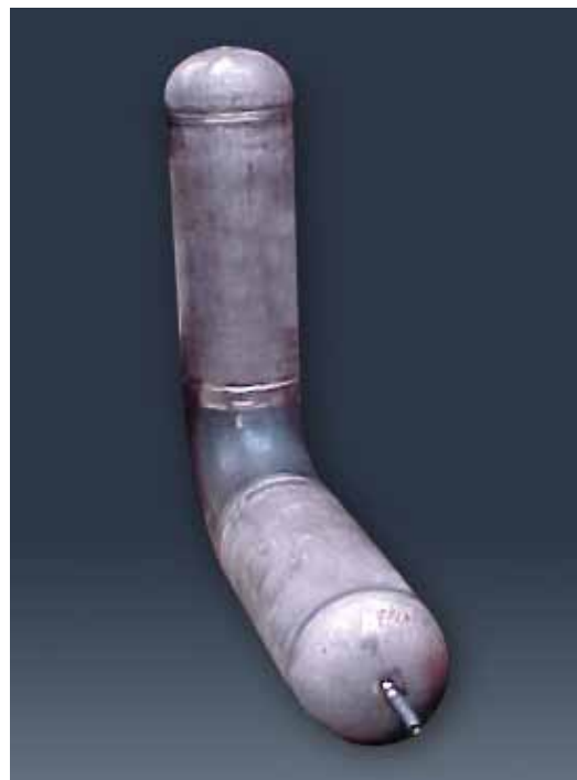
Northrop Grumman Shipbuilding has procured seamless Alloy 625 elbow piping for CVN 78 that was manufactured using a newly identified closed-die, cold forming technique that saves raw material costs. National Technical Systems photo
