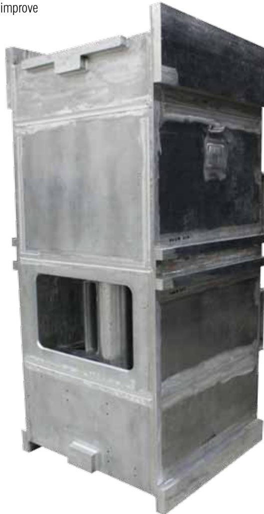
NMC optimized manufacturing approaches used for the Advanced Gun System pallet in DDG 1000, resulting in $5.3 million manufacturing cost savings per hull, as well as a weight reduction that will improve safety and survivability. CTC photo
