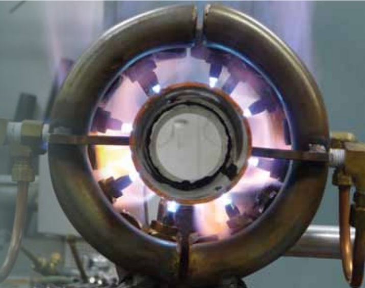
NMC is developing a prototype flame brazing system that will reduce labor and production costs for CVN and VCS. CTC photo
